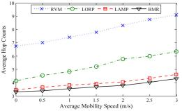
Figure 7: The average hop counts in different protocols for the different average mobility speed.
