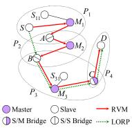
Figure 1: An example of routing paths constructed by RVM and LORP between the source *S* to the destination *D*.
